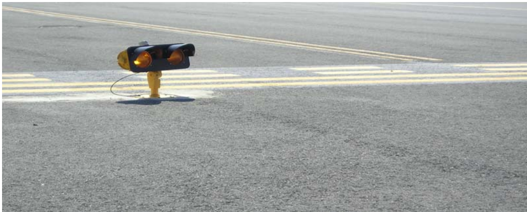
Figure 6. Picture of an Elevated Runway Guard Light at Boston Logan
